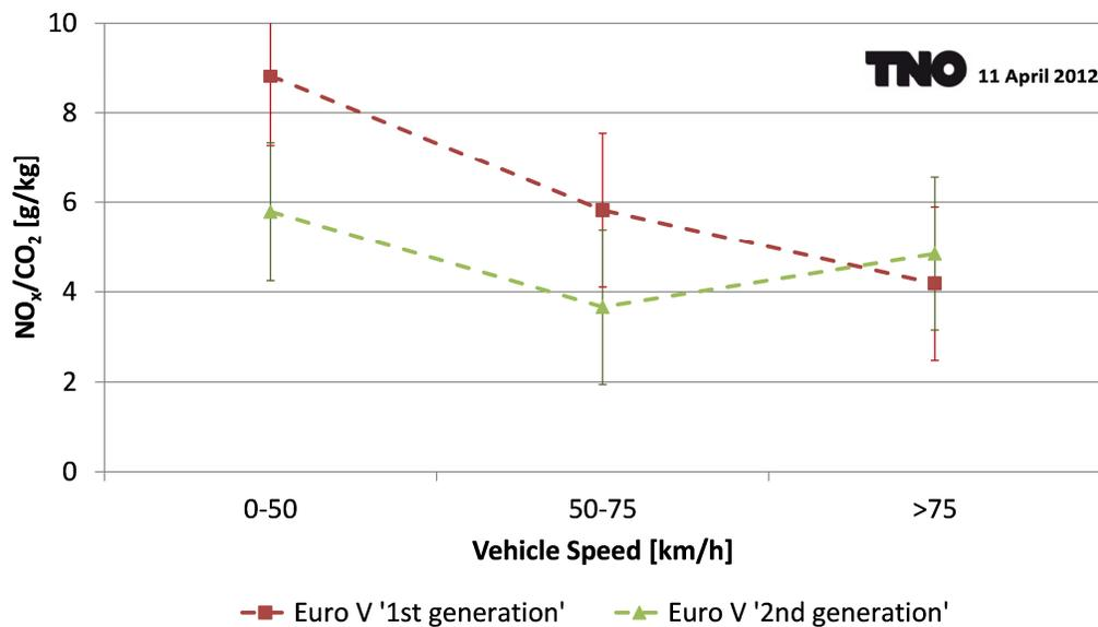
Another cross section of the dataset shows the  $\text{NO}_x$  emissions for individual Euro V and EEV vehicles on diesel and one on LNG (Liquid Natural Gas), see Figure 2.
