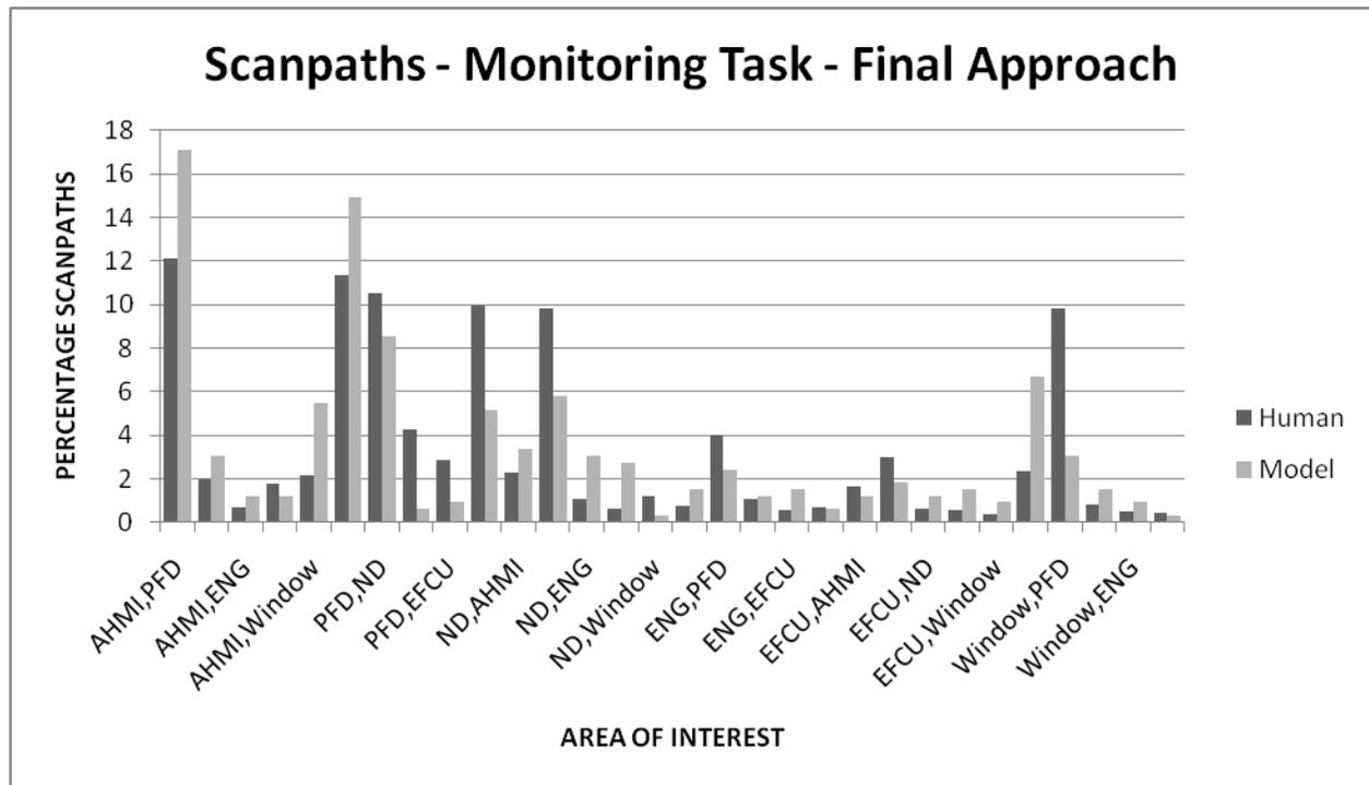
**Figure 6: Comparison of scanpaths between model and human pilots during monitoring task in final approach**
