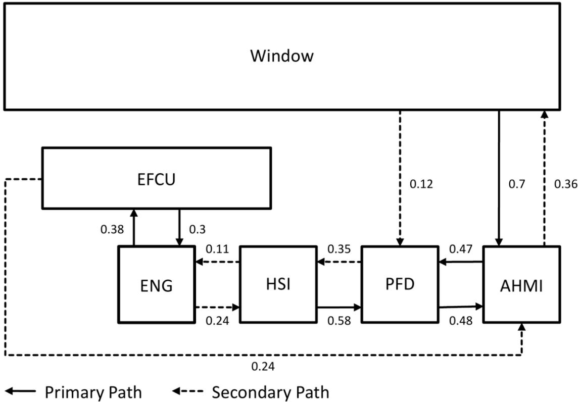
**Figure 2: Scanpaths (primary and secondary) of human pilots during monitoring task while flying in cruise phase (numbers on transitions are transition probabilities)**
