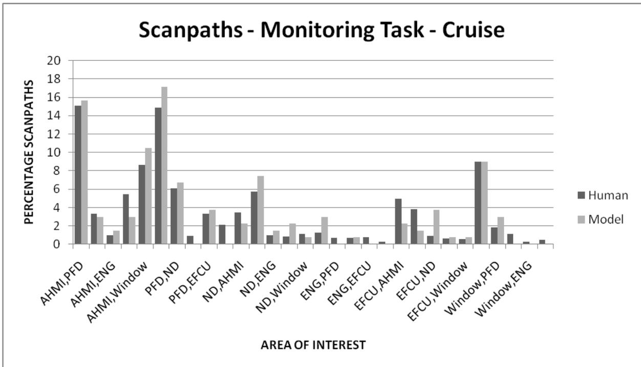
**Figure 4: Comparison of scanpaths between model and human pilots during monitoring task in cruise**
