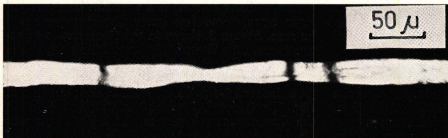
Fig. 9. The same fibre in the polarizing microscope. The Z part in the narrow region of the fibre is not present.
