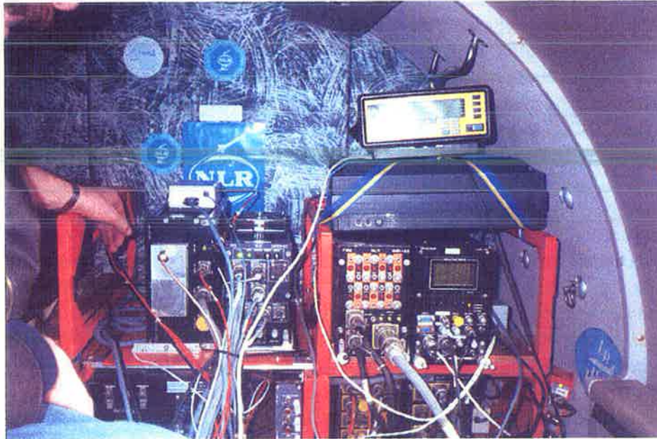
Figure 3.2: The equipment in the aircraft (the Trimble 4000 SSI receiver is at the upper-left side)
