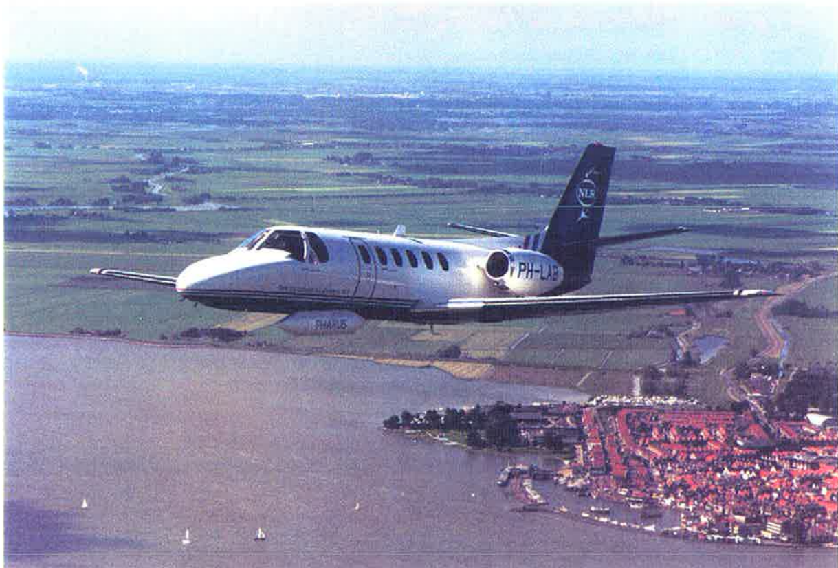
Figure 1.1: The PHARUS SAR system used for this experiment. The radar pod is visible below the cockpit.
