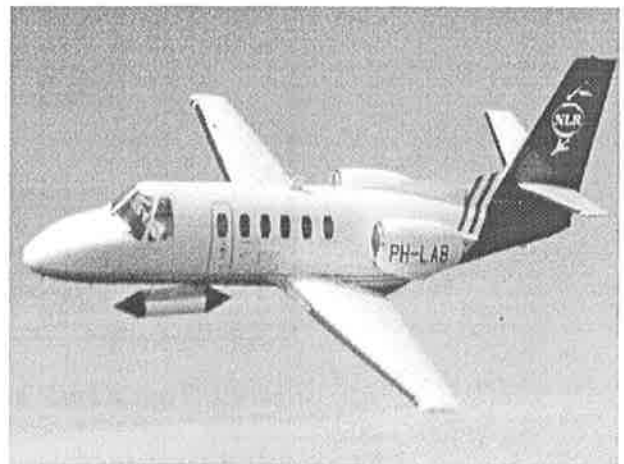
Figure 3: Radar image from Amsterdam (left), Pharus mounted under a Cessna (right)
