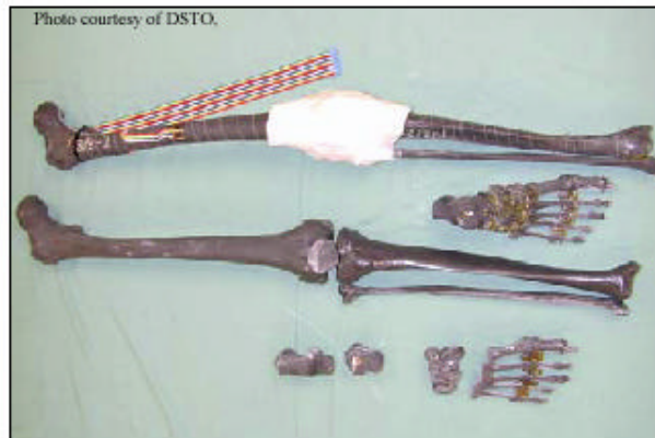
Figure 6 Frangible Surrogate Leg – bone structure (Pictures courtesy of DSTO, Australia)
