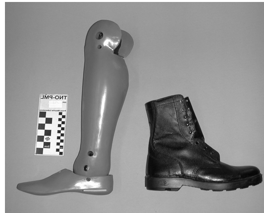
Figure 2 The Netherlands Mechanical Leg (Courtesy TNO PML, Netherlands)
