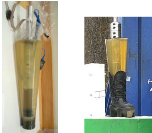
Figure 8 Simplified Lower Leg (Courtesy of DRDC, Canada and DGA, France)
