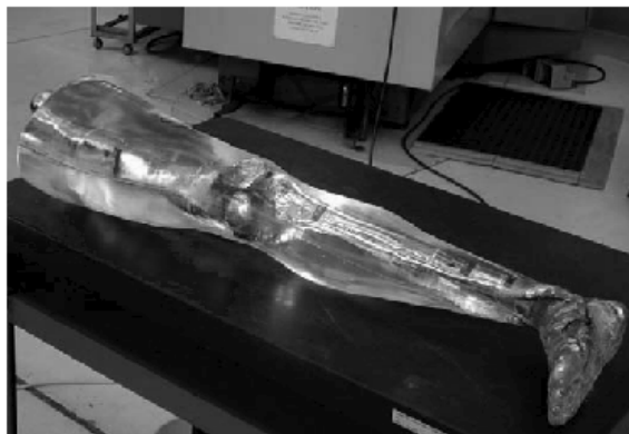
Figure 7 Frangible Surrogate Leg (Pictures courtesy of DSTO, Australia)
