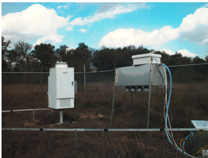
Figure 2 Precipitation collector and equipment for taking air samples at the Speulderveld location.
