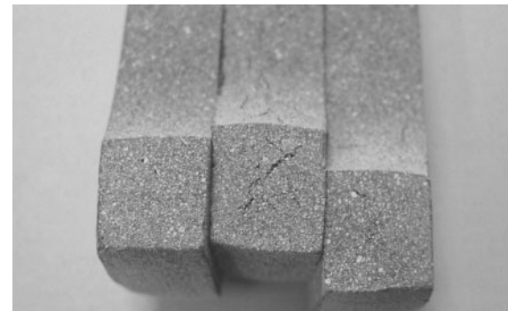
FIGURE 12b. Magnification of one of the samples showing cracks after thermal heating.
