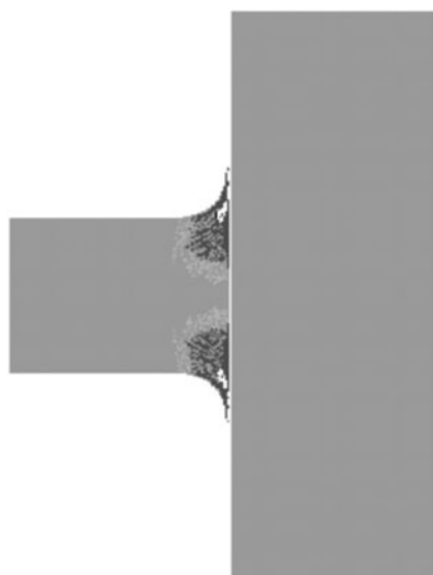
FIGURE 5b. Numerical simulation of HU-43 impacting steel at a velocity of 150 \text{ ms}^{-1} .
