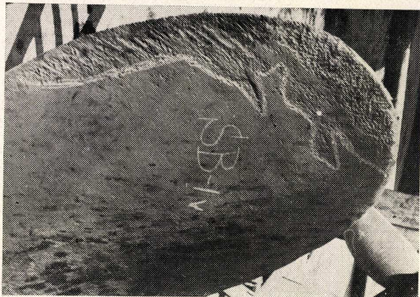
Cavitation and erosion of a ship's propeller.
