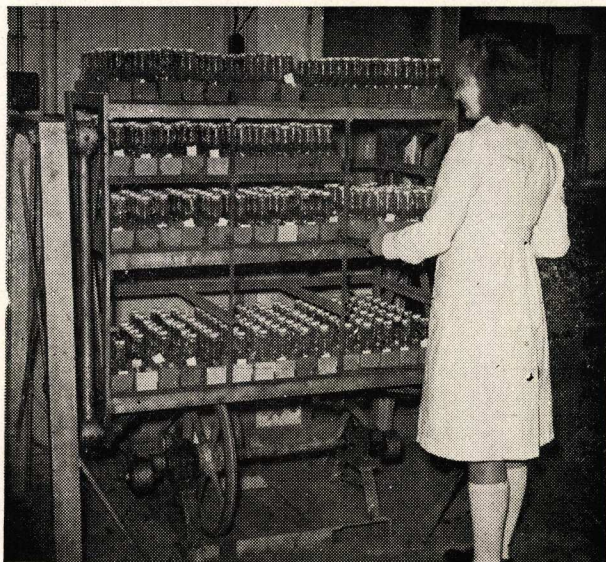
Vibrating machine used to extract soil for measurement of phosphate and potash content.
