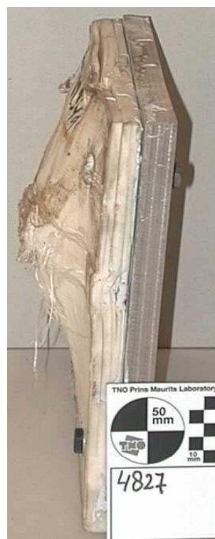
Figure 16: 20 mm Dyneema liner after perforation
