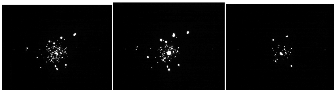
Figure 18: First (left), second (middle) and third (right) witnessplate of a steel armour target
