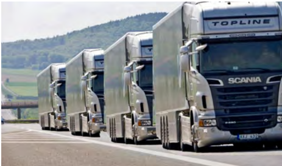
Fig. 4. Platooning technology will eventually allow pelotons beyond two vehicles (Source: Road Safety GB 9 )
