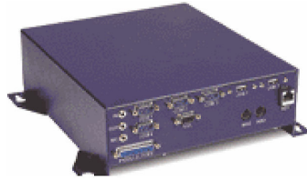
Figure 104: example of an Industrial PC that can be used as Edge Server
