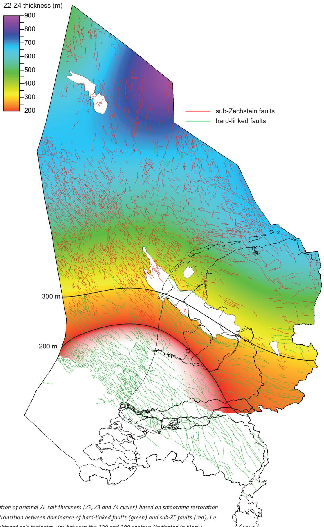
Fig. 8. Thickness distribution of original ZE salt thickness (Z2, Z3 and Z4 cycles) based on smoothing restoration as described in text. The transition between dominance of hard-linked faults (green) and sub-ZE faults (red), i.e. between thick- and thin-skinned salt tectonics, lies between the 200 and 300 contour (indicated in black).
