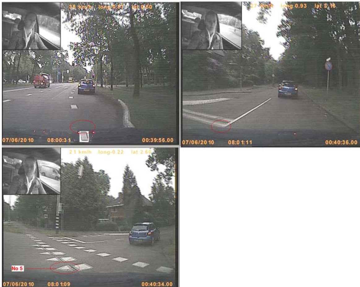
Figure 47. Upper left: reference point for entering the Area of Interest. Upper right: reference point for leaving the Area of Interest. Lower left: reference point for entering the Conflict Area.
