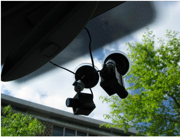
Figure 41. Two camera's mounted with suction mounts behind the rear view mirror.
