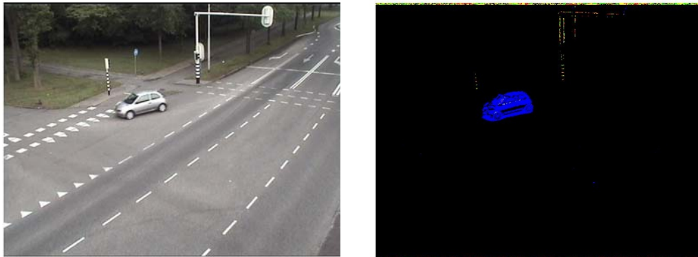
Figure 35. Left picture: Car turning right. The car is the moving object that has to be detected. Right picture: By subtracting the video frame from the background estimation, the foreground pixels will be visible (in blue), because the background remains the same.
