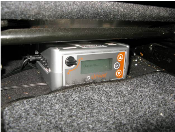
Figure 42. The Data Acquisition System installed under the driver's seat
