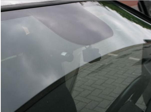
Figure 43. Tinted foil applied to the windscreen to obscure the camera mounts.
