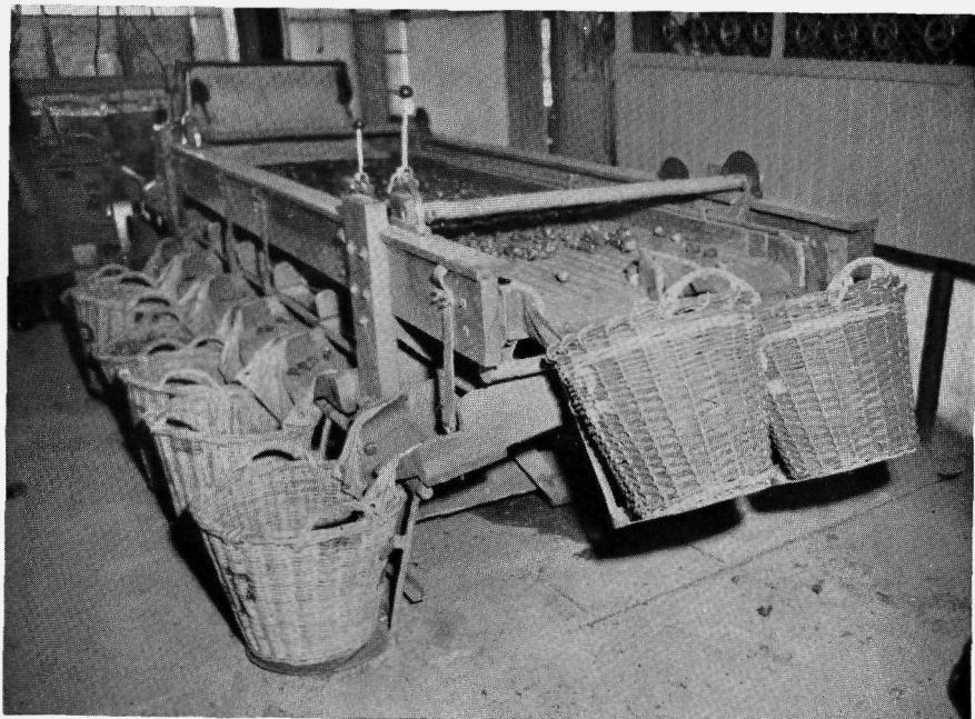
MECHANIZATION: BULB-SORTING MACHINE (Courtesy of Zonneveld & Philippo N.V.)
