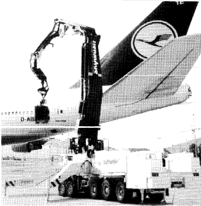
Figure 25 Large scale manipulator for aeroplane cleaning (Courtesy Dornier GmbH).
