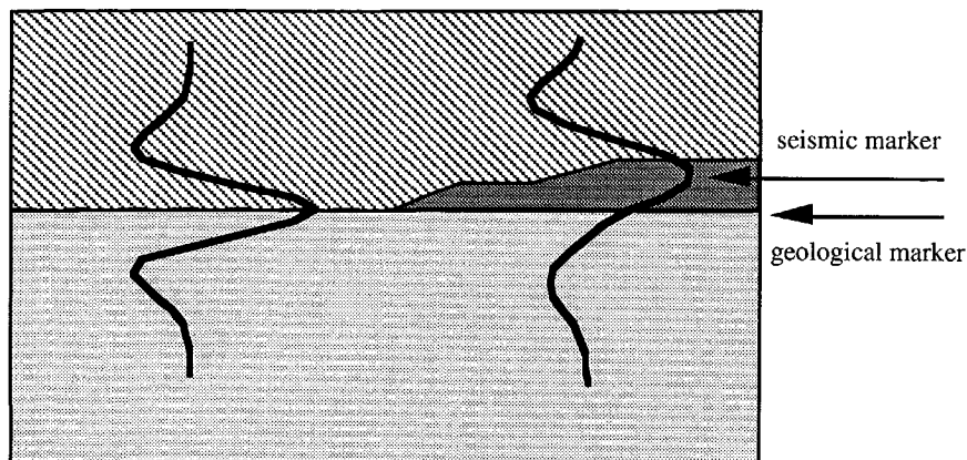
Fig. 7.1 Two types of reference horizons; geological markers and seismic markers. The position of the seismic marker can change laterally relative to the position of the geological marker.
