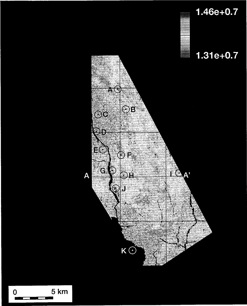
Fig. 6.7 Neural network lateral prediction grid for the weighted average impedance of the Wustrow formation.
