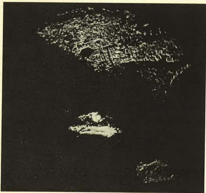
Fig. 4. Radar picture of Bergen (Norway) 0.86 mm radar, d/r \sim 1/150 , S \sim 1800 m.
