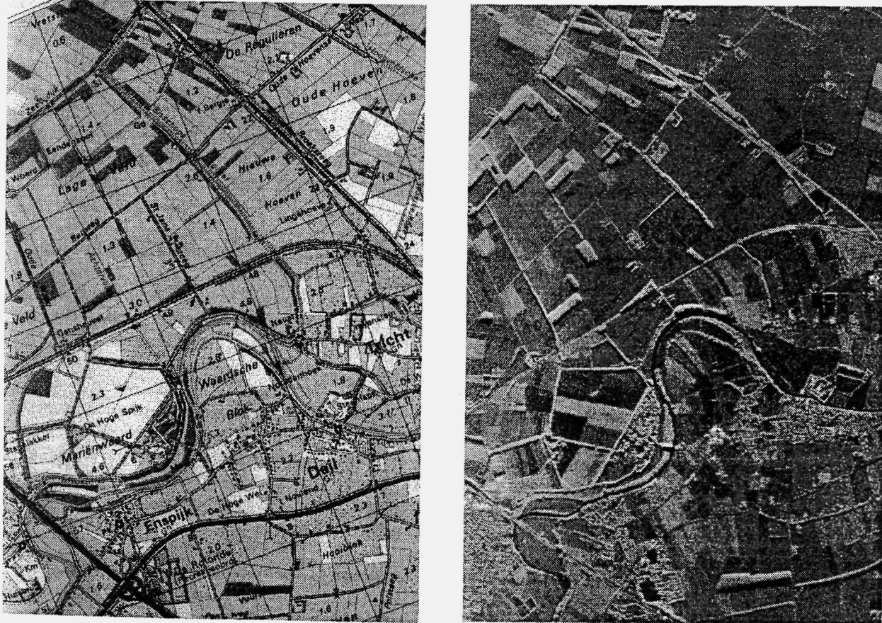
Figure 2. PHARUS image (right) recorded during the first testflight on 22 September 1995. The image shows the Betuwe area in The Netherlands. It is a composite image of the HH and VH channels. Resolution 3 meter, flight altitude 5 km. On the left a part of a topographic map is given, showing the same area.
