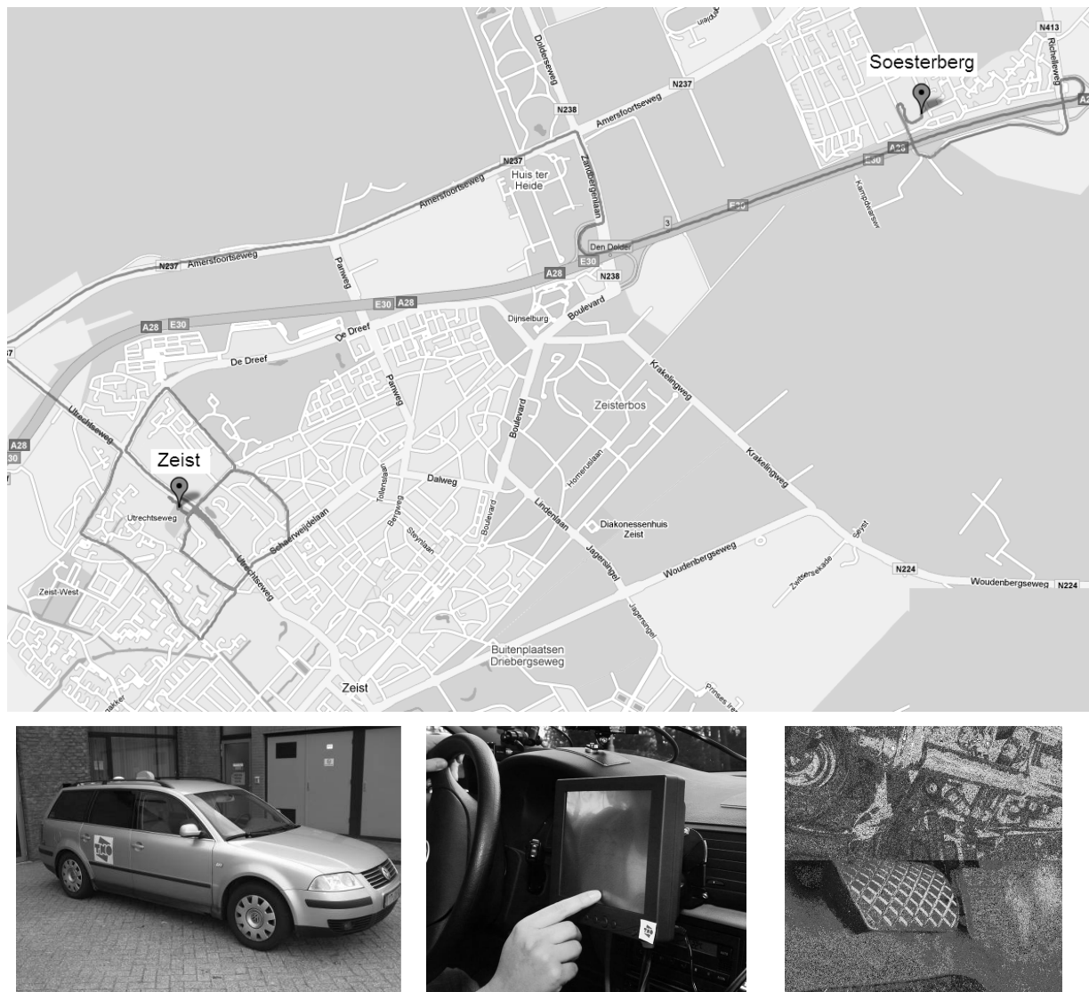
Fig.1. The route (Google maps©), instrumented car, the screen and the haptic gas pedal
