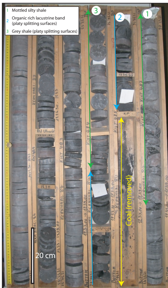
Figure 7.3 Core-photograph of a lacustrine band (RLO-LB 2). The mottled sediment (1) below the coal is well developed, as well as the organic-rich section (2) on top of the coal (lacustrine band). The white labels indicate the sample locations.
