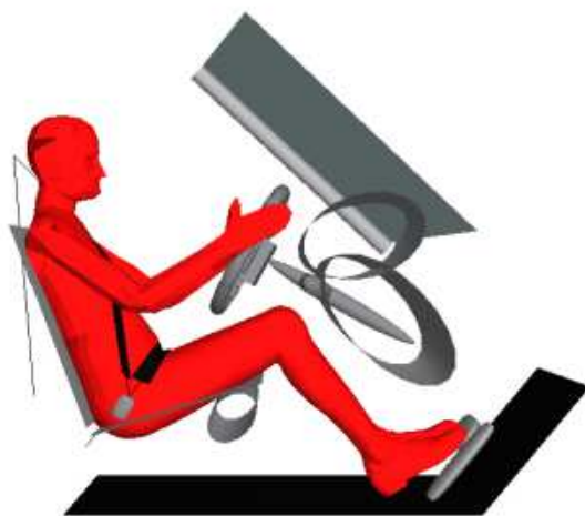
Figure20. Position of active (red) and passive (green) model at onset of the frontal impact simulations of the small car.
