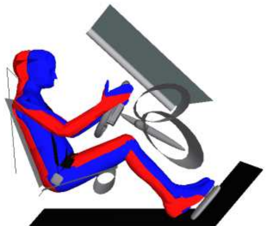
Figure23. Position of the active model with (blue) and without (red) preceding braking at 1000 ms of the frontal impact simulations of the small car.
