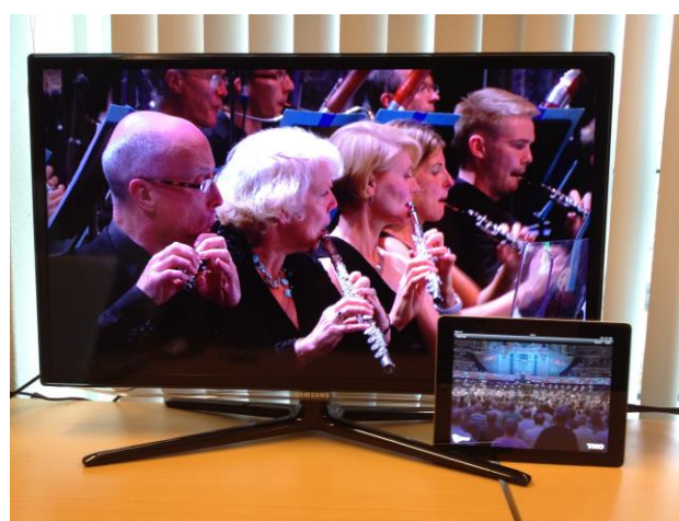
Figure 5: DVB-S stream on TV, synchronized with a video panorama of the same event running on a tablet
