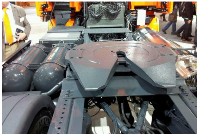
CNG and LNG storage on one vehicle
