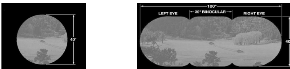
Figure 5: Comparison of the rather narrow NVG field-of-view to the much roomier Panoramic NVG field-of-view.
