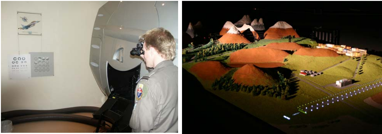
Figure 1: Stage 2 of the current NVG training. On the LEFT demonstration of the reduced visual acuity and contrast sensitivity with F4949 NVG's. On the right the AMST terrain board, demonstrating a variety of NVG effects like halo's, inability to look into shadows, confusion of colored lights, etc. These demonstrations focus on the reduced NVG visibility of objects more than NVG illusions. The DISO simulator shown in the left image is the primary tool for SD training, requiring active participation of the course participants.
