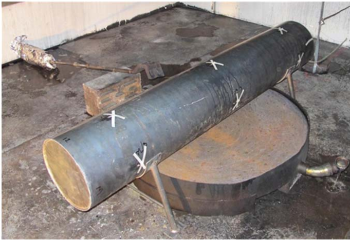
Figure 3 Dummy ordnance position directly over the fuel pan in Position 1.
