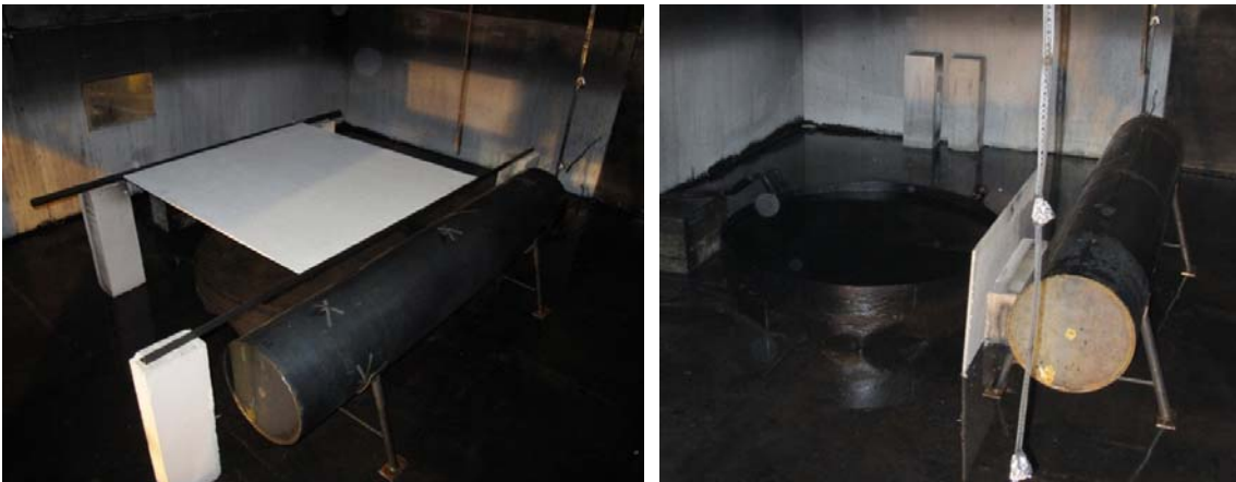
Figure 4 Promatect calcium silica board obstruction used when the fuel pan was in Position 2, horizontal (left) and vertical (right).
