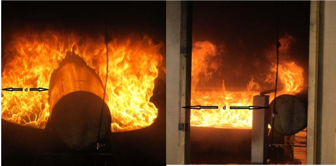
Figure 10 Difference in effective flame thickness with the two different fuel pan positions
