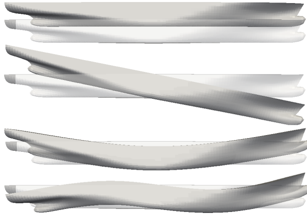
Figure 1.2: Generalised modes for a ship with two flexible modes.
