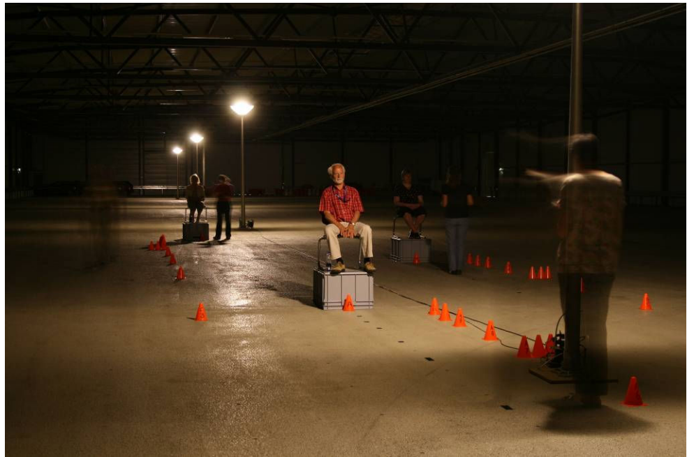
Figure 21 Overview of the experimental set-up, with the light poles, three locations of the target persons (sitting on a platform) and the subjects (standing) assessing recognition of the target person faces.
