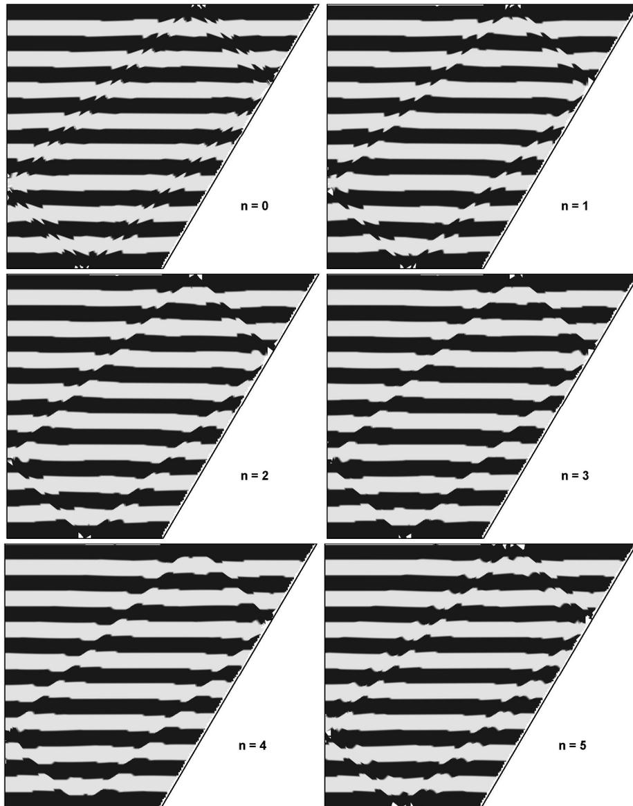
**Figure 4.14:** Example of iteratively defined travelling wave solution  $\Psi(x, z, t)$  for ‘surface sloshing’ boundary condition;  $p_a(x) = \sin(x\pi/2)$ . Here the associated displacement is shown by artificial ‘dye’ bands for times  $n = 0, \dots, 5$ , with  $t/T_w = n/12$ .
