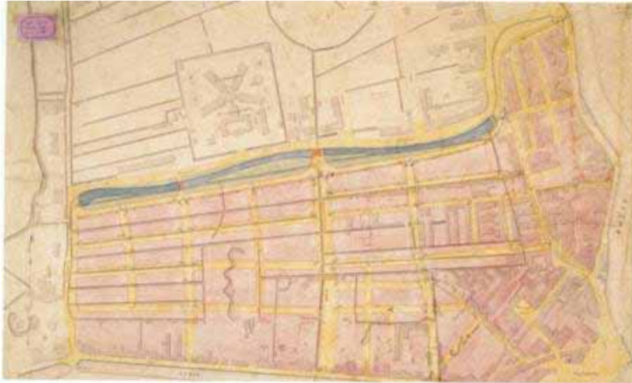
Picture 4.16 Oostblommersdijkpolder with proposed urban blocks (in pink) drawn over the polder pattern, from which the subsidence of houses can be predicted. It shows the sharp contrast between the open space and large-scale houses along the singel with the dense areas with smaller houses and streets behind it.
