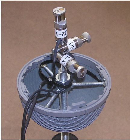
Figure 2: 3D acoustic vector sensor.
