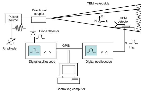
**Figure 3** Measurement setup for detector tests
