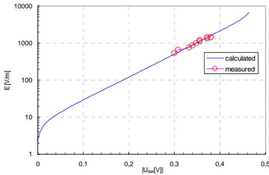
**Figure 5** Comparison of measured and calculated results for  $f = 1.2$  GHz
