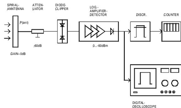
**Figure 1** Block diagram of the first development stage of the HPM detection system
