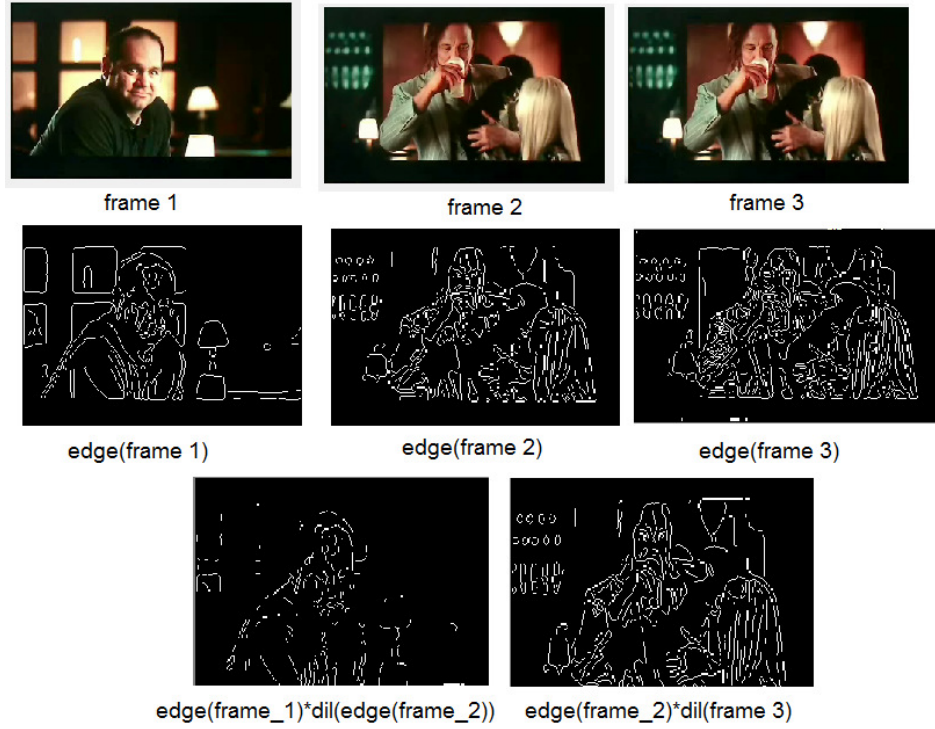
Figure 2.10 A graphical illustration of the static scene change feature using edge maps
