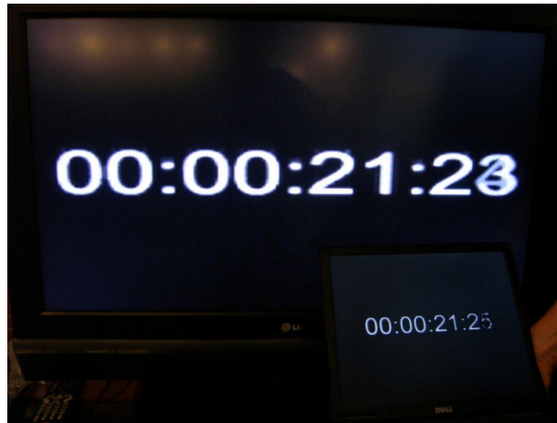
Figure 2.2 Play-out difference measurement of input lags
