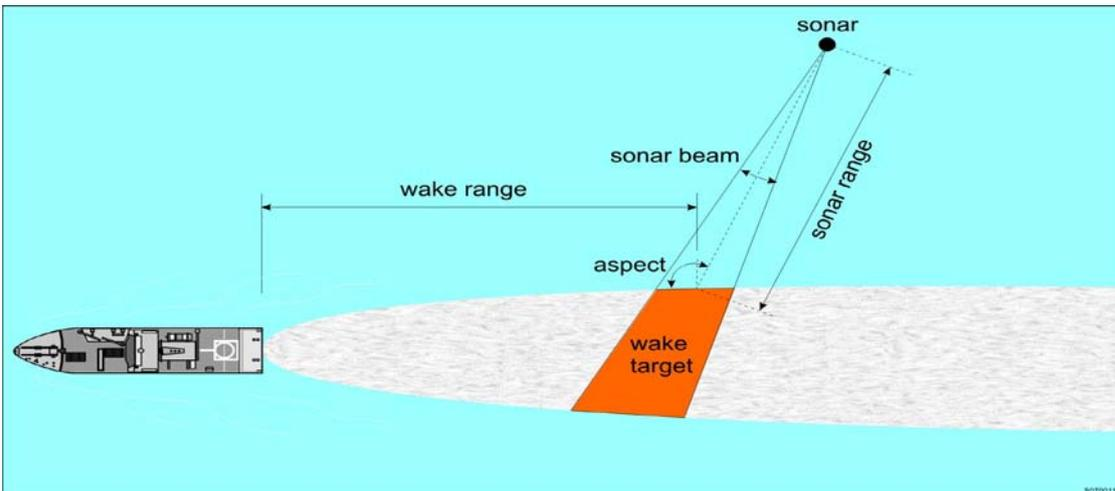
Fig.1 Sonar detection scenario with wake
