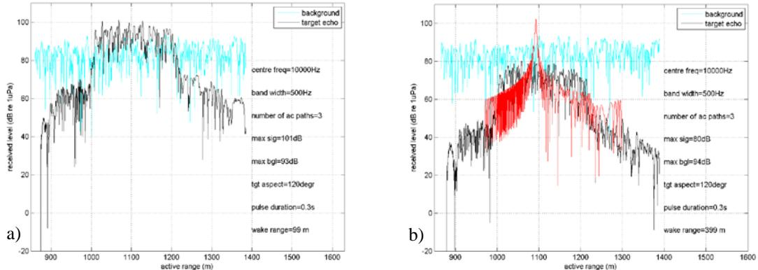
Fig.3: modelled echo structure of wake at 10 kHz a) at wake range 100 m b) at 400; in red a 0 dB point target.
