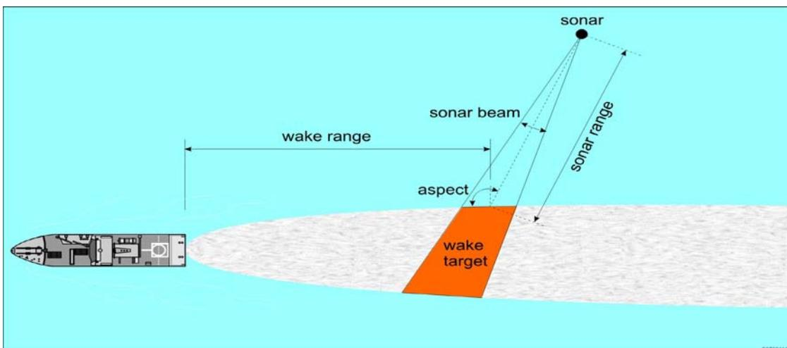
Fig.1 Sonar detection scenario with wake
