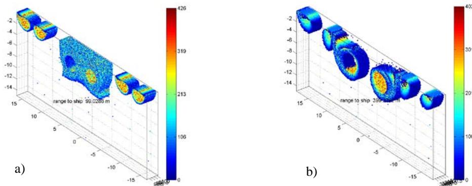
Fig.2: Cross section of wake a) at 100 m wake range (behind ship) b) at 400 m.
