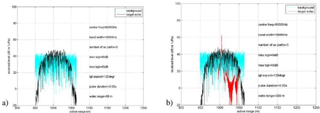
Fig.5: modelled echo structure of wake at 60 kHz a) at wake range 100 m b) at 400; in red a 0 dB point target.
