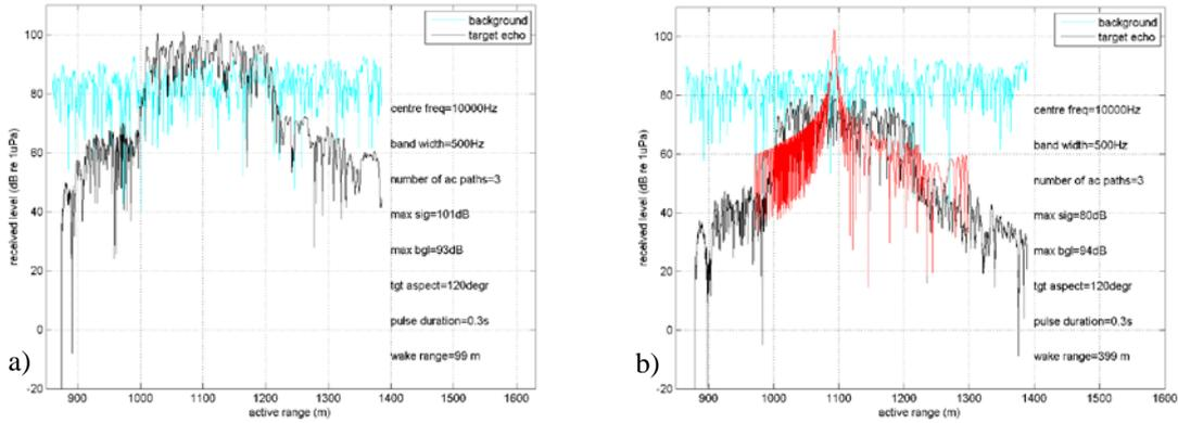
Fig.3: modelled echo structure of wake at 10 kHz a) at wake range 100 m b) at 400; in red a 0 dB point target.
