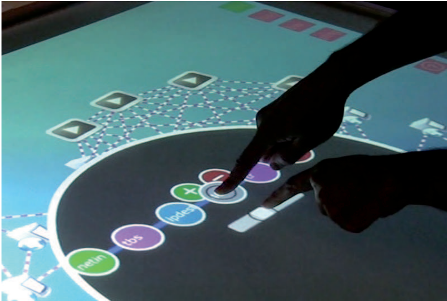
Figure 10. A closer view on the sampler modification interface. The sampling percentage is changed with the slider.
