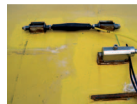
Underwater sensors, mounted on the pile
