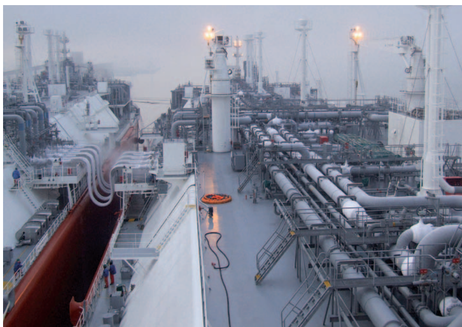
Offshore transfer of LNG using hoses by Gutteling, courtesy of Exmar
