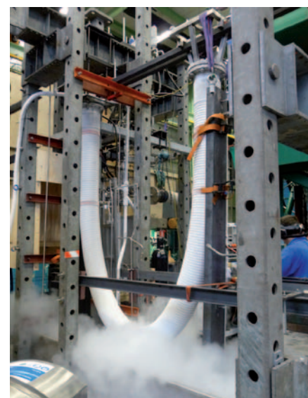
Cryogenic bending test of the hose
