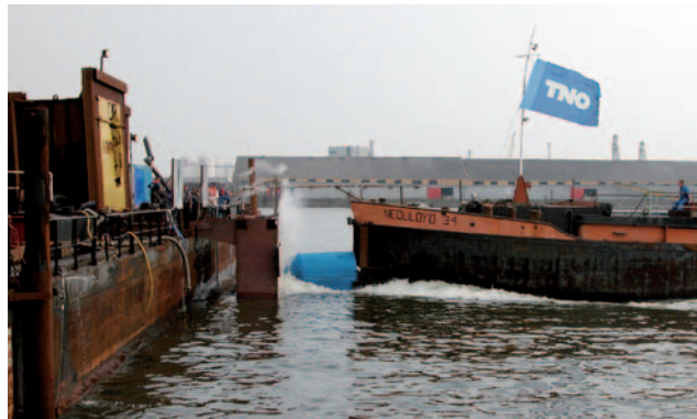
Full-scale testing of impact-resistant side walls
