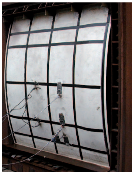
Test on a light-weight and affordable explosion-resistant structure
