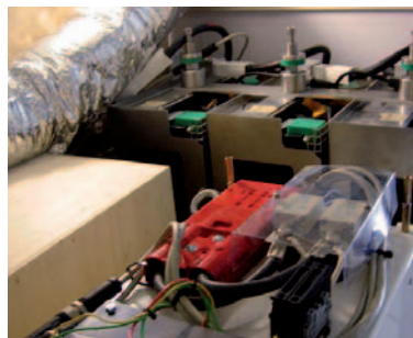
Battery system test arrangement for the Ethereal
