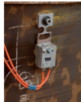
Above-water sensor, mounted on the pile
