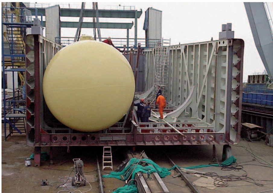
Gas tank in a hull with impact-resistant side walls
