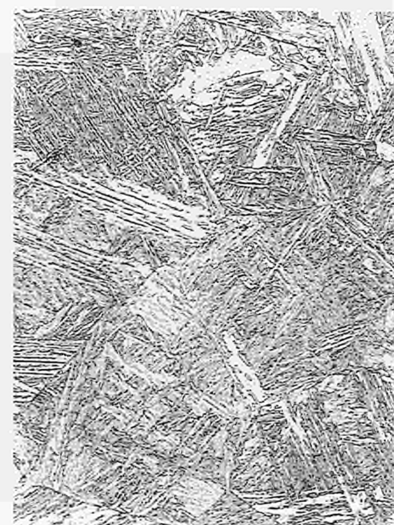
Fig. 4.106 Microstructure of simulated specimens of material N a: \Delta t(800-500) = 7 sec. b: \Delta t(800-500) = 12 sec. c: \Delta t(800-500) = 20 sec. d: \Delta t(800-500) = 50 sec. M=x500
