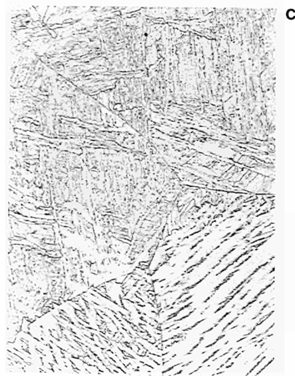
Fig. 4.111 Microstructure of simulated specimens of material QT Simulation conditions: 1350°C/12 sec. a: as simulated b: +1h 530°C c: + 1h 560°C d: +1h 590°C M=x1000
