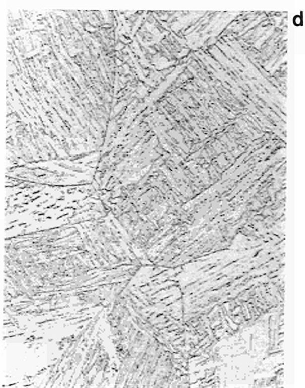
Fig. 4.111 Microstructure of simulated specimens of material QT Simulation conditions: 1350°C/12 sec. a: as simulated b: +1h 530°C c: + 1h 560°C d: +1h 590°C M=x1000
