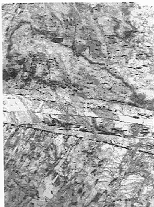
Fig. 4.116 TEM pictures of extraction replica's and thin foils of material TM, simulation condition: 1350°C/12 sec. a: replica, +1h 530°C b: replica, +1h 590°C c: thin foil, +1h 530°C d: thin foil, +1h 590°C a,b: M=x2000 c: M=x6000 d: M=x4000
