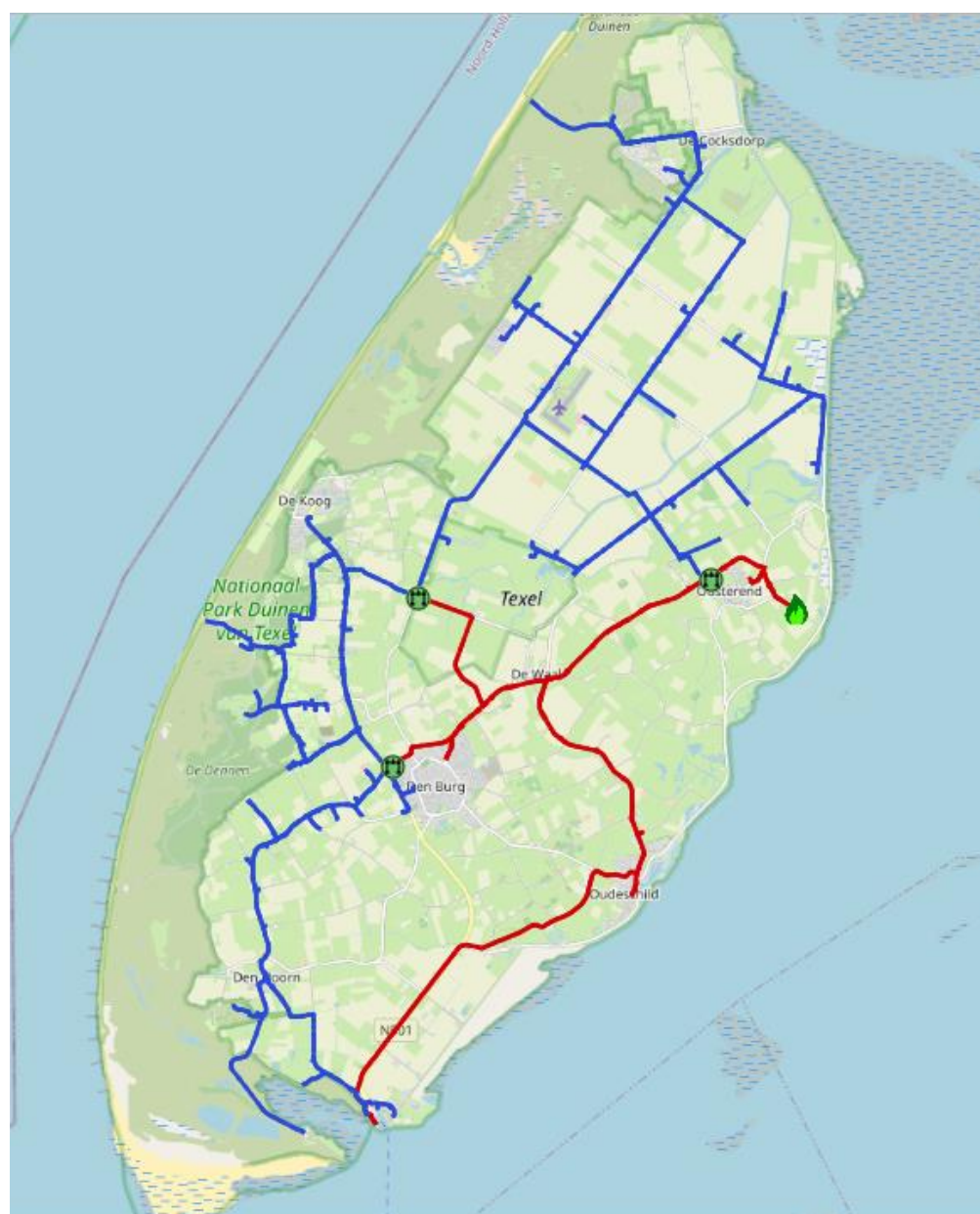
Figure 6. Texel gas network pipelines: 3 bar (blue line) and 8 bar (red line).
