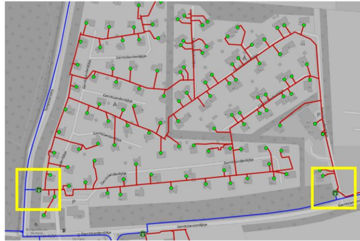
Figure 9. The customers located in the blue square of Figure 8. The yellow squares indicate the pressure reducing stations from 3 bar to 100 mbar.
