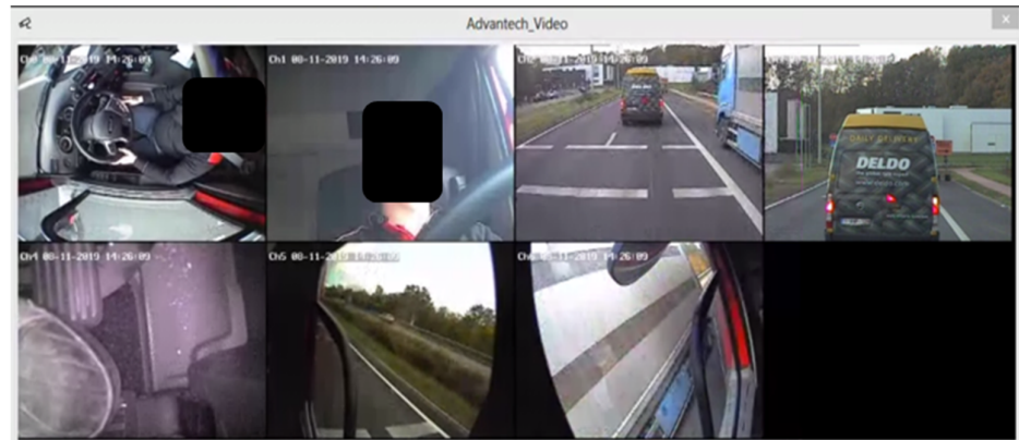
Figure 22: Camera views of the installed cameras. Clockwise from top left: top down cabin view, driver view, forward view wide, forward view narrow, pedals view, right side mirror, left side mirror.
