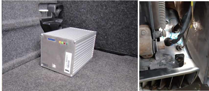
Figure 16: Smart Emissions Measurement System (SEMS), with sensors in the exhaust.
