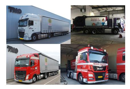
Figure 2: Tested vehicles with Euro VI step A to C certified diesel engines and one heavy-duty dual fuel engine (below left).
