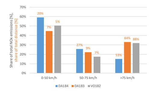
Figure 7: The share of the  $NO_x$  emissions of the total emissions per speed interval of the tested vehicles with a step D certified engine. A large share of the total  $NO_x$  (45 to 59%) is emitted at the low speed range whereas the most of the kilometres (53 to 88%) are driven in the higher speed range.
