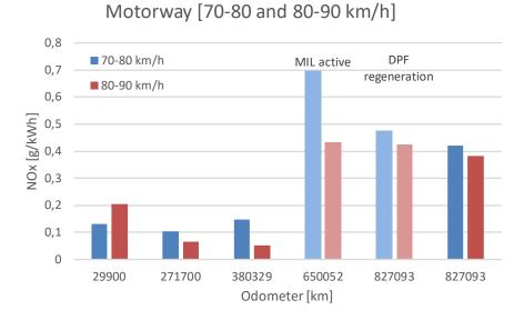
Figure 11: NO<sub>x</sub> in speed bins at motorway speeds. The trips have comparable motorway driving with a fully warmed up drive train and aftertreatment. Trips are driven with the same total vehicle weight (tractor, semi-trailer and payload).
