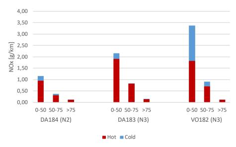
Figure 8: Contribution of cold starts in total emissions per speed interval:  $NO_x$  emissions when the engine has a coolant temperature <70 °C (Cold) and >= 70 °C (Hot).
