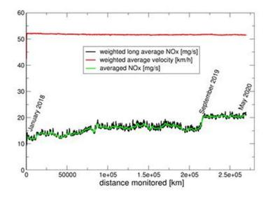
Figure 13: A statistical approach weighing influences of cold starts, velocity, engines speed and CO<sub>2</sub> emissions give the corrected NO<sub>x</sub> emissions in mg/s over time. This reveals a step in NO<sub>x</sub> emissions from about 15 to 20 mg/s around September 2019. The owner mentioned an indication at the dashboard of an Adblue error that occurred in September 2019. The Adblue dosing unit and two NO<sub>x</sub> sensors were replaced.
