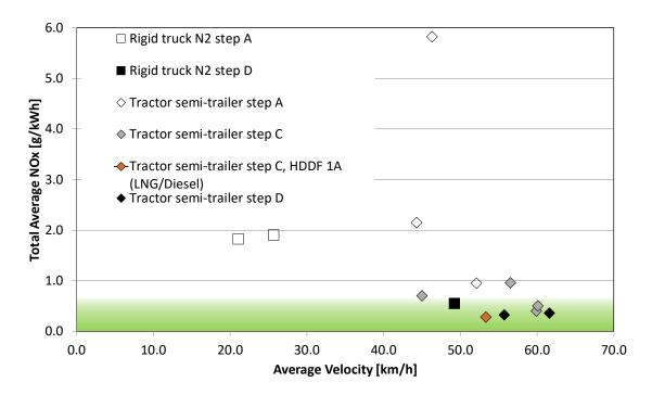
Figure 5: Total average NO<sub>x</sub> emissions versus average speed for all vehicles tested with SEMS in normal daily operation. The upper side of the green area represent a NO<sub>x</sub> emissions level of 0.69 g/kWh, which is the limit of the conformity factor of 1.5 expressed in gNO<sub>x</sub>/kWh (1.5x0.46=0.69 g/kWh) for the formal ISC test. Individual vehicles can't be compared as operation differs from vehicle to vehicle.
