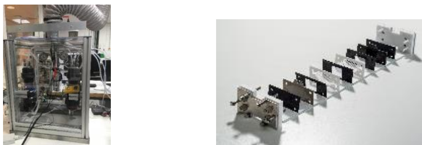
Figure 2: Low pressure continuous flow reactor & TNO's electrochemical cell design
