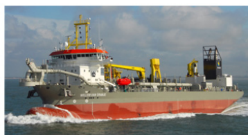
Trailing suction hopper dredger
