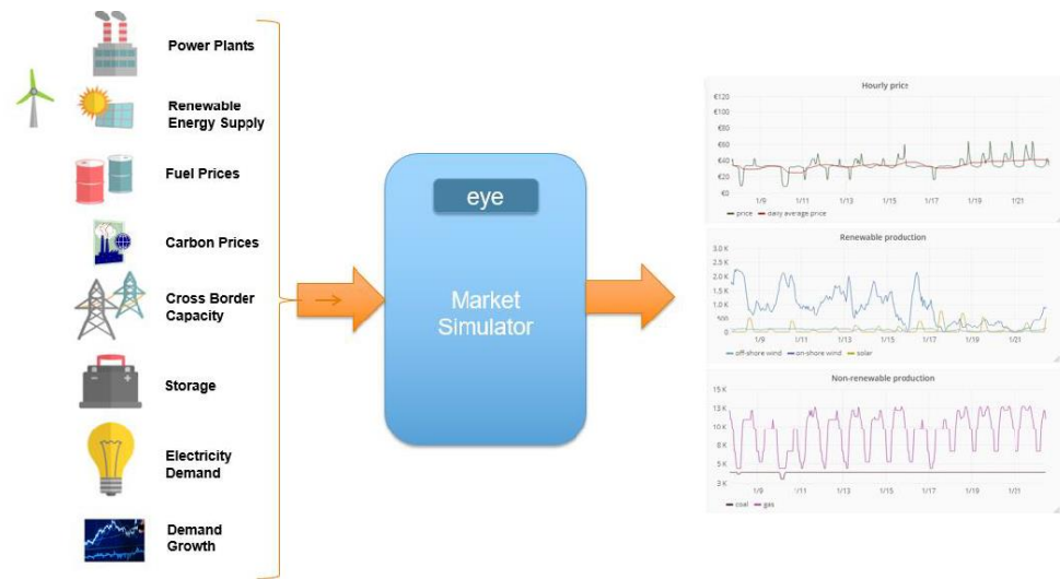
Figure 2.18: Overview of EYE simulator with inputs: models of demand and supply bid behaviour, and outputs such price and production/consumption profiles of individual assets.
