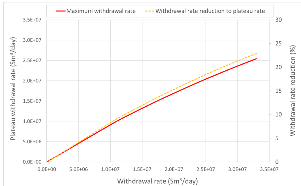
Figure 3.10: Plateau withdrawal rate of 3 months versus the maximum theoretical withdrawal rates estimated for the case of hydrogen in the Grijpskerk reservoir at 393 bar pressure (maximum working pressure), for a large range of initial wellhead pressure and using a 7-inch (ID) production tubing (see also Figure 3.8). The yellow line shows the percentual reduction of the plateau withdrawal relative to the maximum initial theoretical withdrawal rate.
