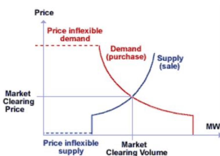
Figure 2.17: Electricity clearing mechanism to set the hourly electricity price, based on required electricity volume per hour. Including inflexible supply (e.g. wind energy) and inflexible demand (e.g. CCGT with base load heat supply)
