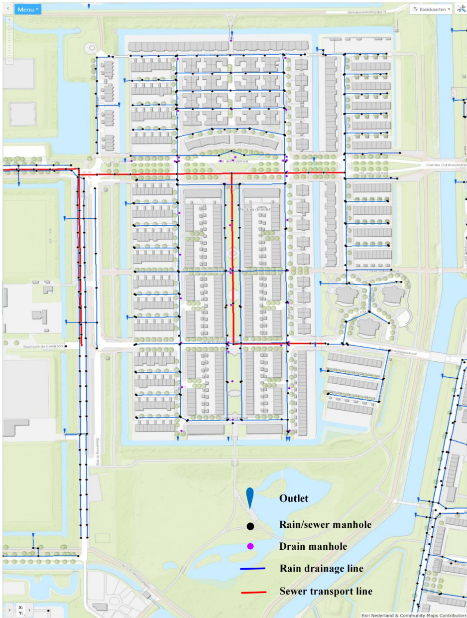
Figure S3.1.2 Rain water drainage system and the sewer system
