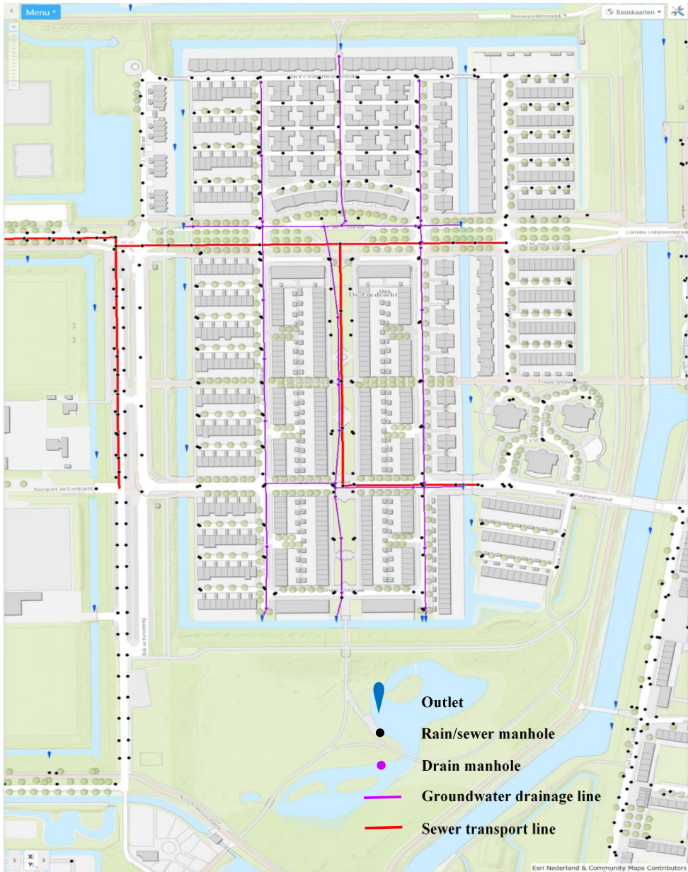
Figure S3.1.1 Groundwater drainage system and the sewer system
