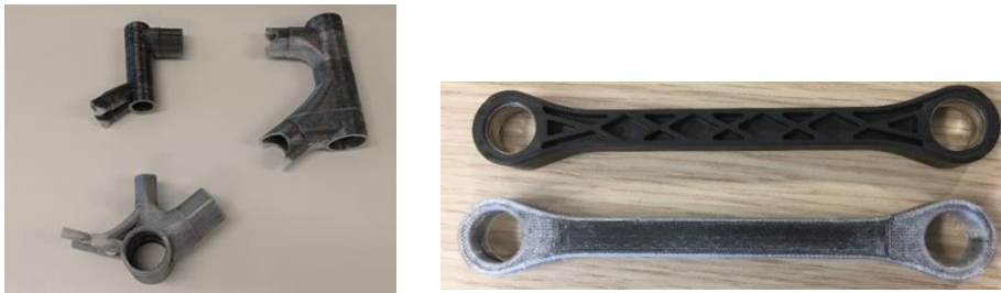
Figure 2: 3D printed parts with continuous carbon fiber
