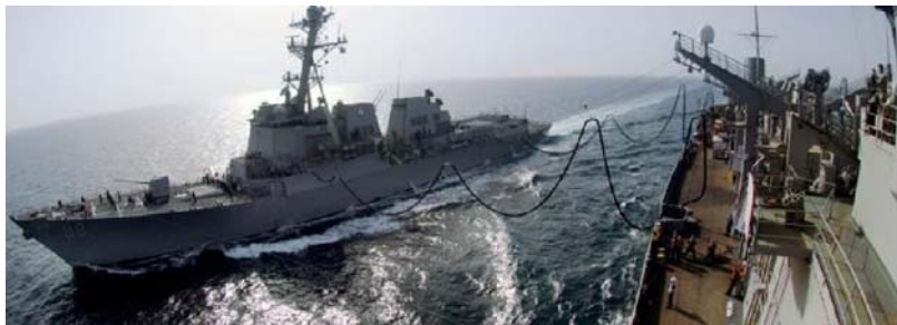
Figure 9: Line transfer bunkering at sea [12]
