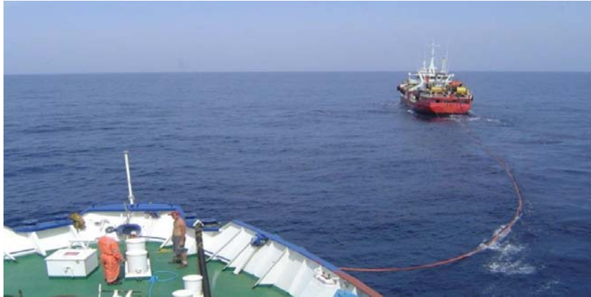
Figure 8: Stern line bunkering at sea [12].
