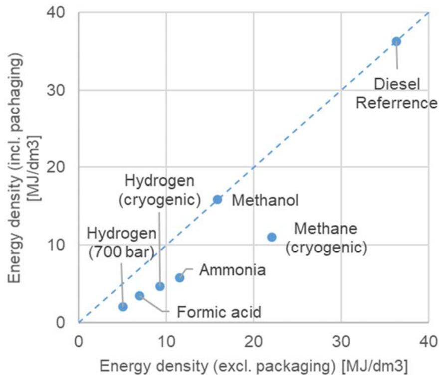
Figure 6: Energy density of different fuel types (TNO (2019))
