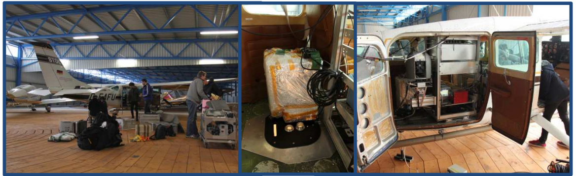
Figure 1: SPECTROLITE breadboard tested in DLR airplane campaign over Berlin.
