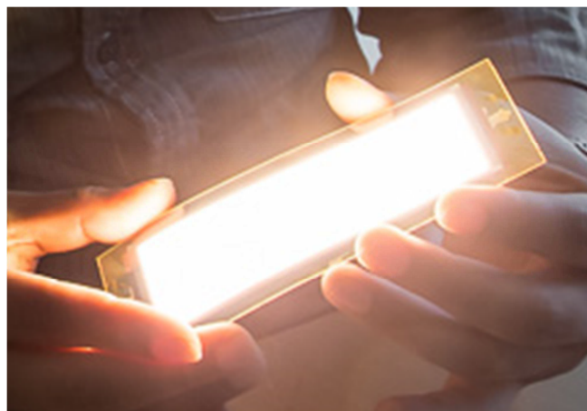
High brightness ( 10\,000\text{ cd/m}^2 ) evaporated OLEDs on flexible plastic (PEN)/water barrier/anode foils, with shelf lifetimes of >5 years.
