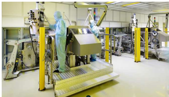
Innovative roll-to-roll facility for flexible photovoltaics on polymer or metal foils.
