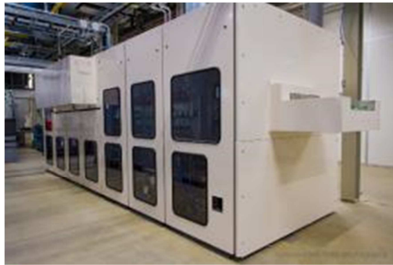
Equipment for fast Atomic Layer Deposition on large area glass substrates (based on TNO invention for spatial ALD).
