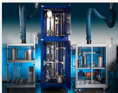
Biphasic reactor for conversion of waste into furans (kg/hr)
